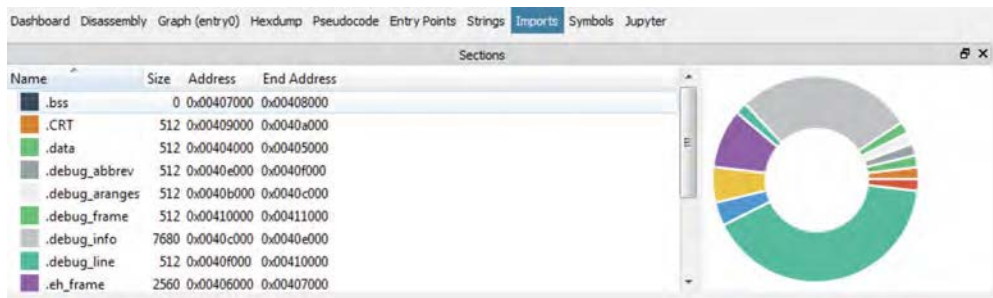
FIGURE 8.5 Portable executable sections
