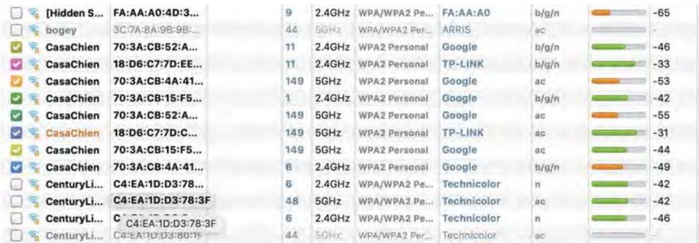
FIGURE 11.4 Multiple BSSIDs for a single SSID
